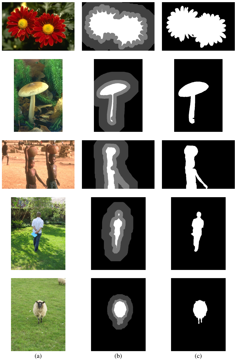
Fig. 2. (a) Original images from the GrabCut dataset, (b) the trimaps providing seed regions, and (c) the original ground truth.
