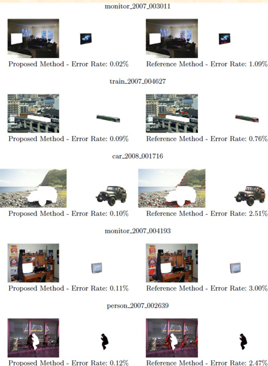
Fig. 5. Images segmentation results by the proposed model with the use of the cut polygon tool and the reference model. Misclassified pixels are highlighted in red. (Color figure online)
